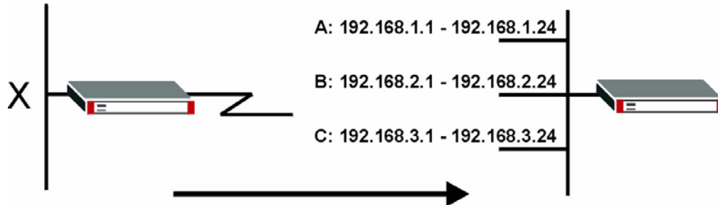
Figure 62 Physical Network and Partitioned Logical Networks
