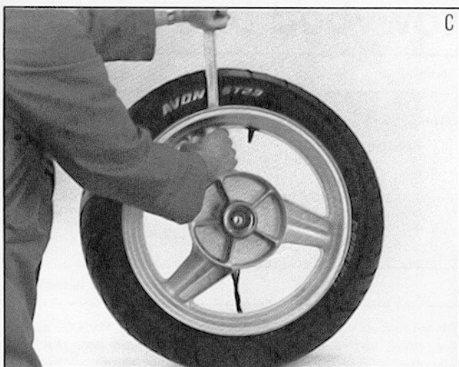
C When first bead is clear, remove tire as shown.
