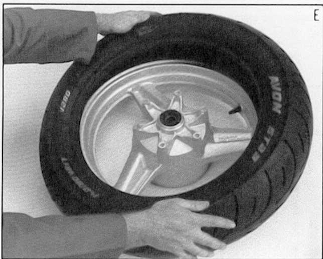
E Work first bead over the rim flange.
