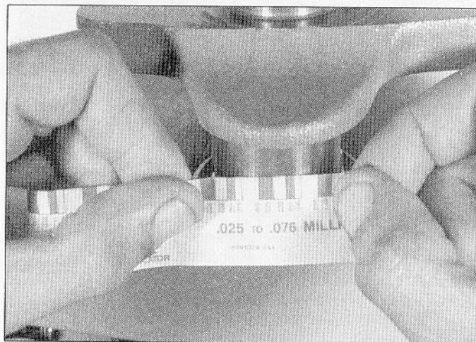
26.13 Place the Plastigage scale next to the flattened Plastigage to measure the bearing clearance
