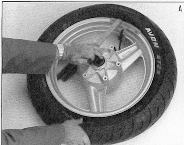
A Deflate tire. After releasing beads, push tire bead into well of rim at point opposite valve. Insert lever next to valve and work bead over edge of rim.
