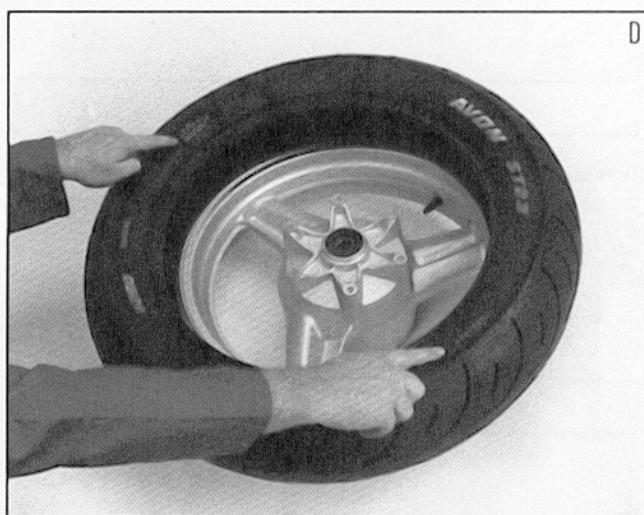
D Before installing, ensure that tire is suitable for wheel. Take note of any sidewall markings such as direction of rotation arrows.
