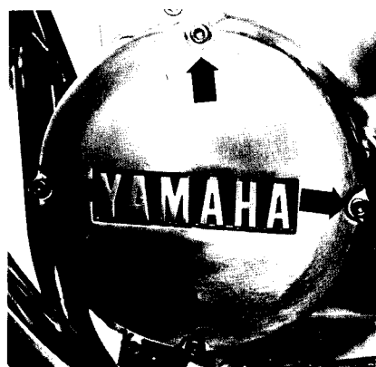
Alternator rotor cover allen bolts
