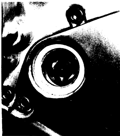
Clutch adjuster screw and locknut
