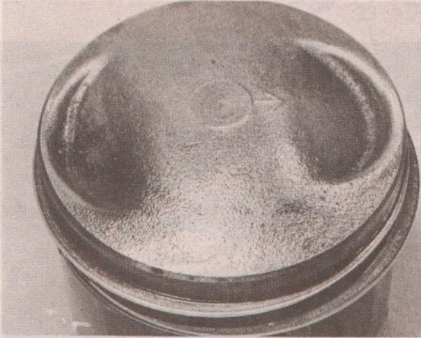
46.4a Arrow on piston crown must face forward
