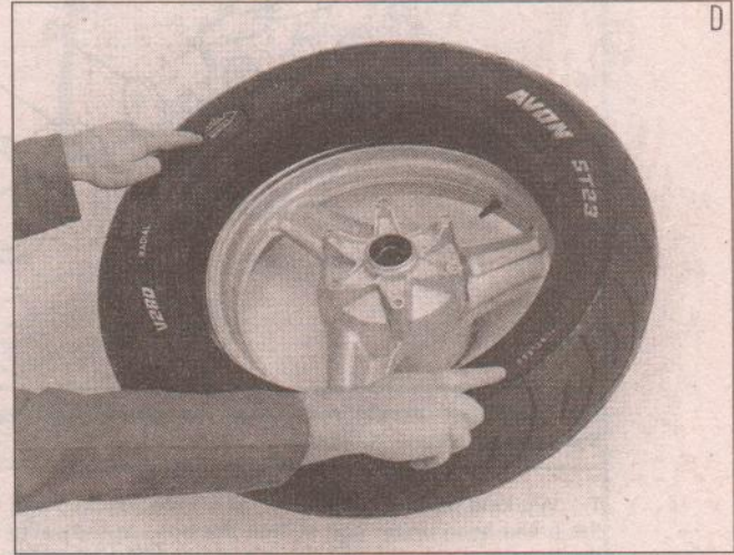
Before fitting, ensure that tyre is suitable for wheel. Take note of any sidewall markings such as direction of rotation arrows.
