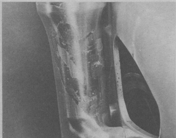
Peeling lacquer on alloy components requires stripping and relacquering to prevent corrosion
