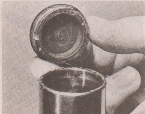
12.1 Remove plastic cap from top of stanchion
