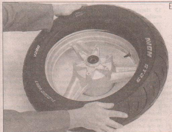
Work first bead over the rim flange.
