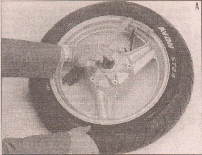
Deflate tyre. After releasing beads, push tyre bead into the well of rim at point opposite valve. Insert lever adjacent to valve and work bead over edge of rim.
