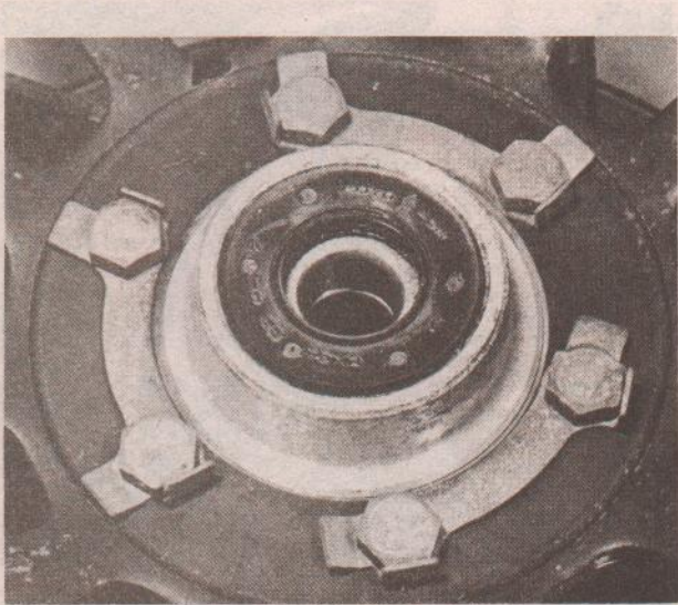
20.4h ... tapping it home until flush with the hub
