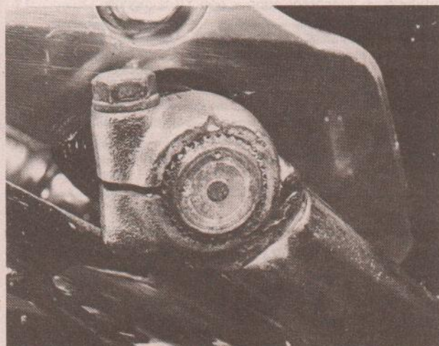
50.13 Align index marks on all control levers or pedals
