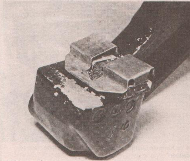
4.2f Note pad guide shims on support bracket lugs
