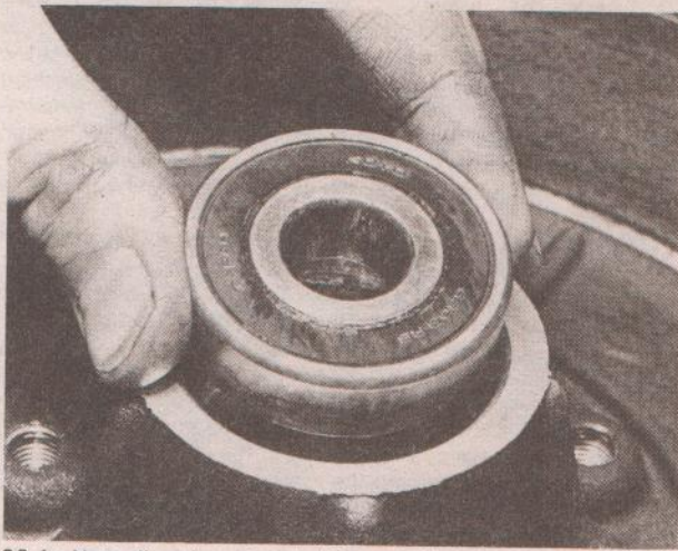
22.1e Note direction of sealed faces on bearings
