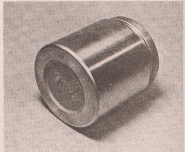
9.7a Examine piston for signs of scoring or wear
