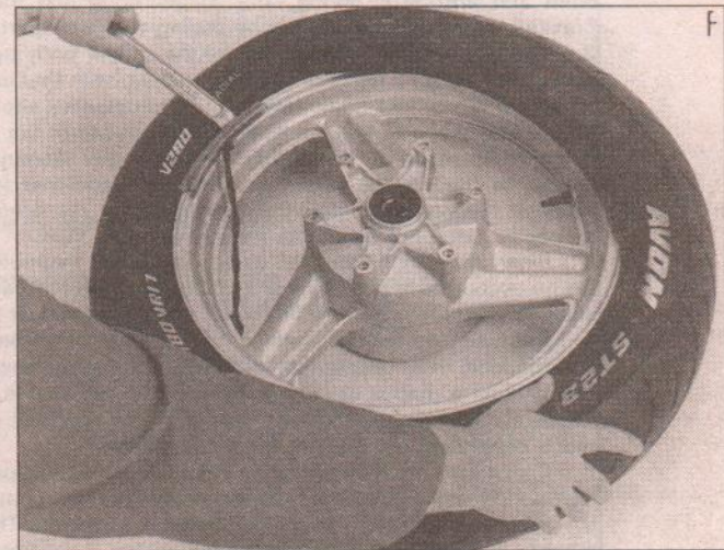
Use a tyre lever to work the second bead over rim flange.
