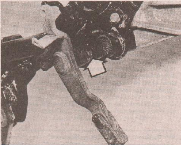
31.1 Link can be displaced inwards to permit greasing
