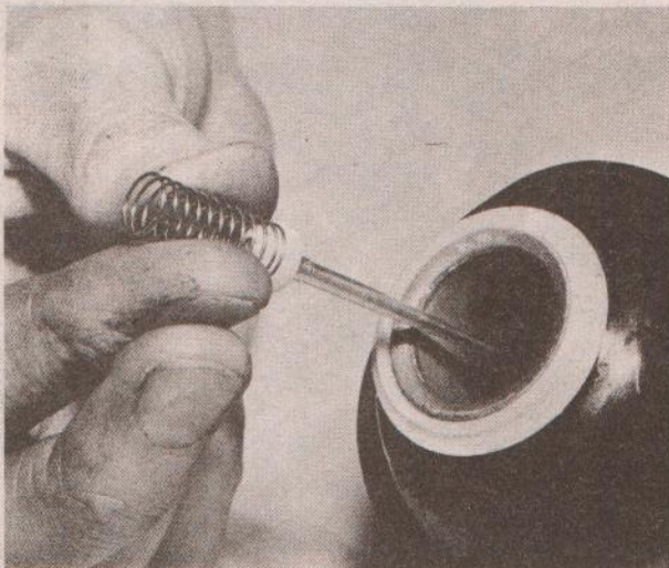
7.8b ... to release the spring and needle
