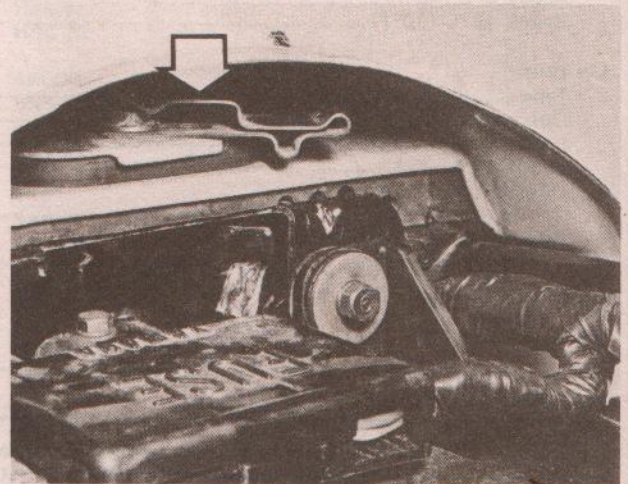
2.1 The tank fixing clip (shown displaced for clarity)
