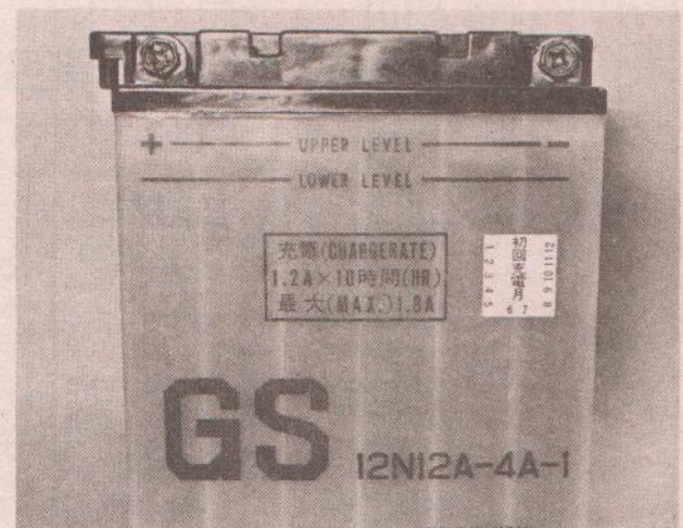
6.2 Battery electrolyte level is visible through translucent case
