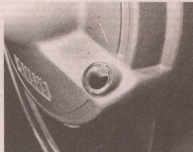
Final drive oil level should just reach the edge of the filler hole
