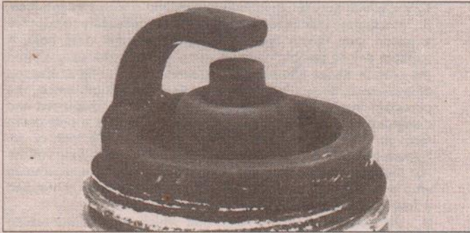
Carbon fouling - Dry, black sooty deposits leading to misfire and weak spark. Caused by an over-rich fuel/air mixture, faulty choke operation or blocked air filter
