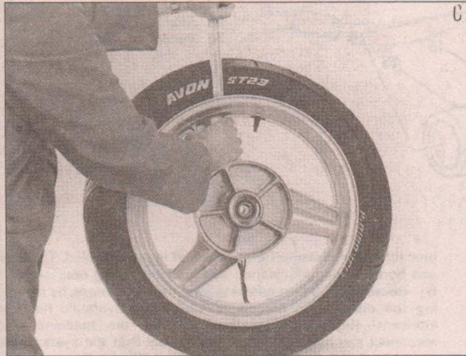
When first bead is clear, remove tyre as shown.
