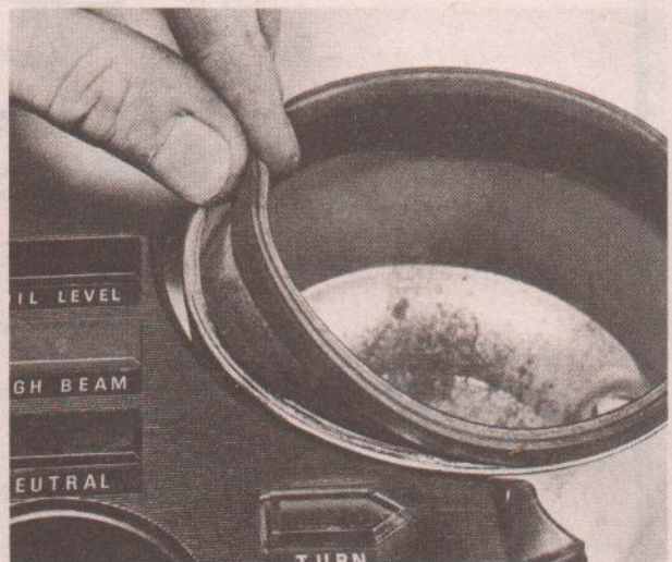
47.4 Note anti-vibration seal around edge of cup
