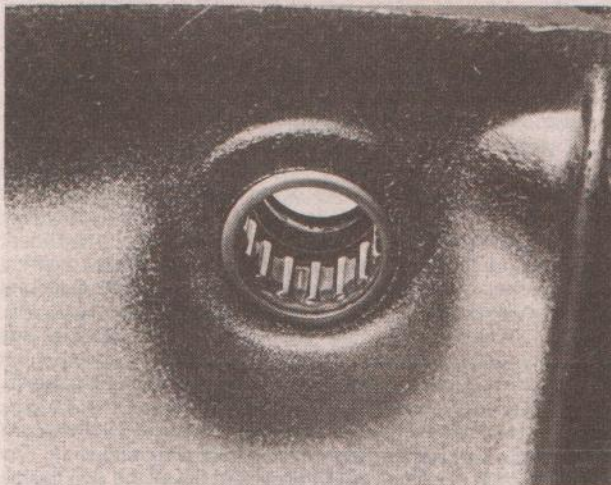
29.7e Lubricate bearings prior to reassembly
