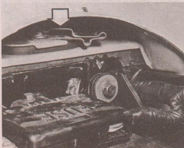
4.4a Release clip or bolt to free rear of fuel tank
