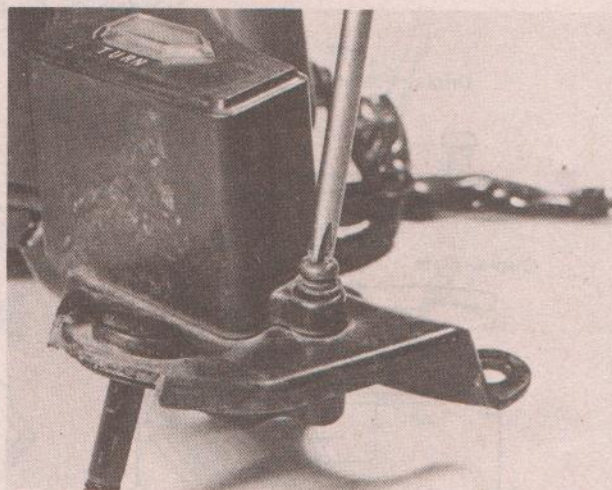
47.1a Warning lamp panel is secured by screws – instrument panel removed for clarity (UK 650)
