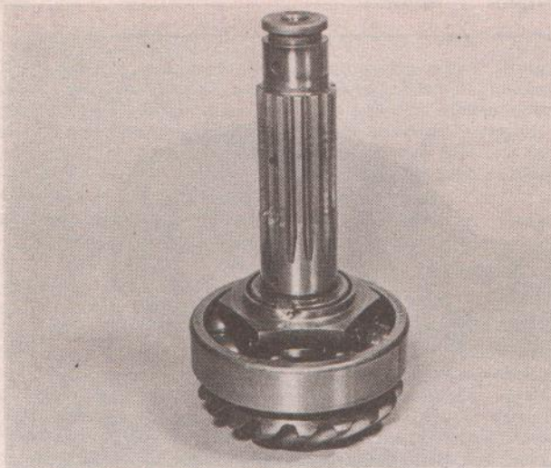
32.6a Bearing is retained on shaft by large nut ...
