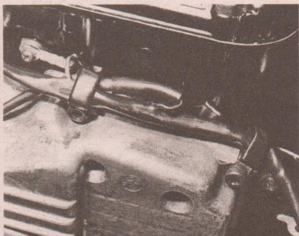
50.9a Cable routing along underside of unit
