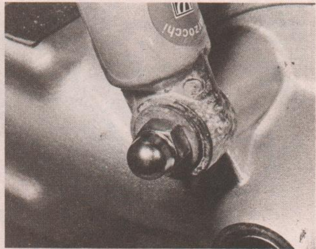
19.4 Remove domed nuts and washers to free the suspension unit lower mounts
