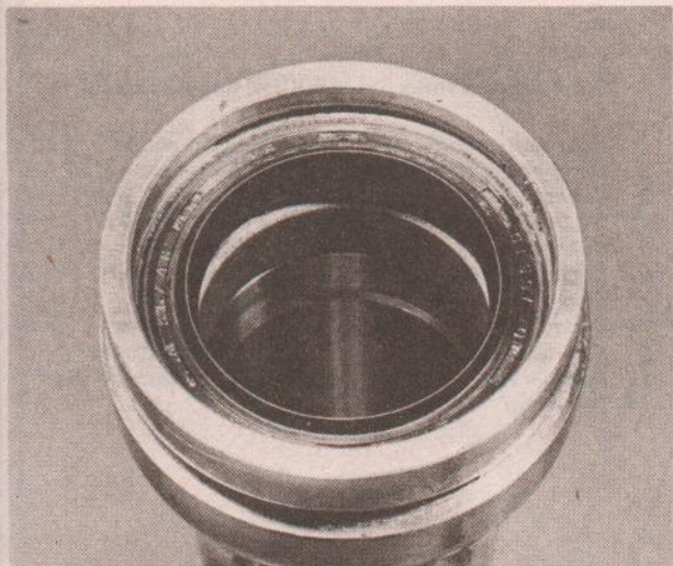
12.8a Check that new seal seats squarely in lower leg
