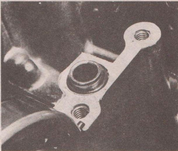
36.1 Fit dowel and a new O-ring to oil passage
