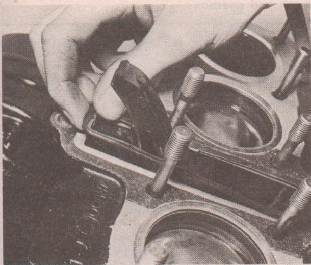
47.2c Do not forget camshaft chain tunnel seal
