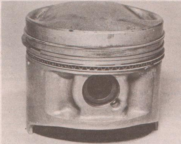
23.2 Check condition of pistons and remove any carbon
