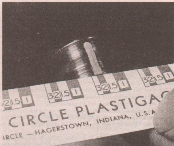
19.4c Measure clearance against scale on edge of pack
