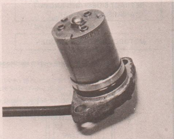
31.2b Switch is sealed unit. Check O-ring condition
