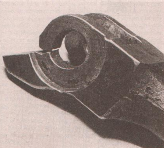
28.1 This stand was cracked and would have failed soon if not spotted. It was repaired by welding
