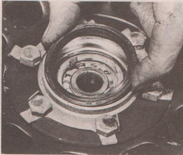
20.4d ... and grease seal
