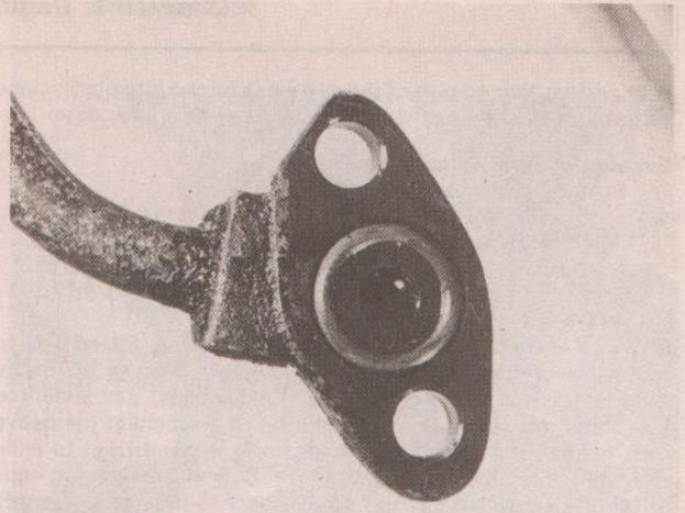
50.5 Use new O-rings on oil cooler unions
