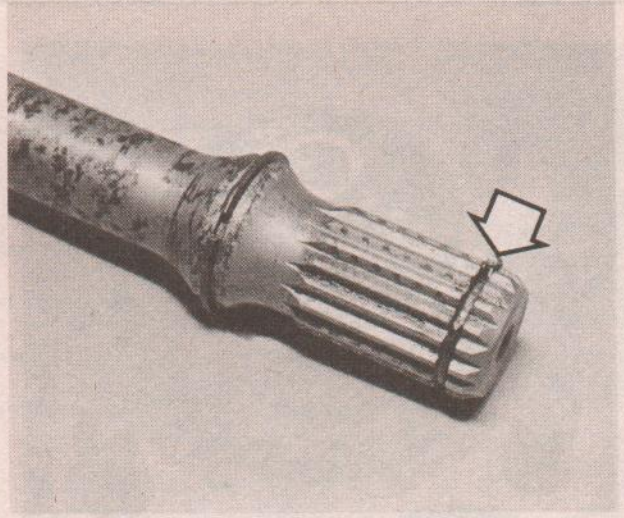
21.2b Spring ring (arrowed) locates in groove in joint
