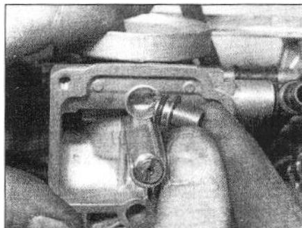
9.5 Install the needle valve seat using a new O-ring
