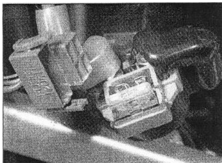
5.3a Disconnect the connector to access the fuse
