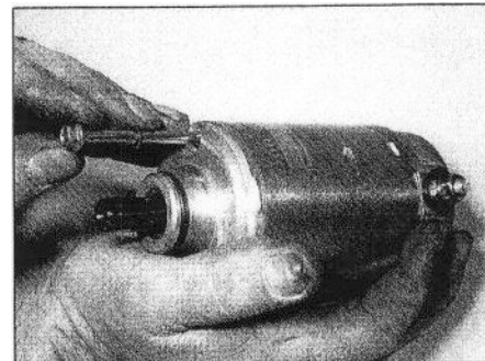
30.21 Install the long bolts using new O-rings
