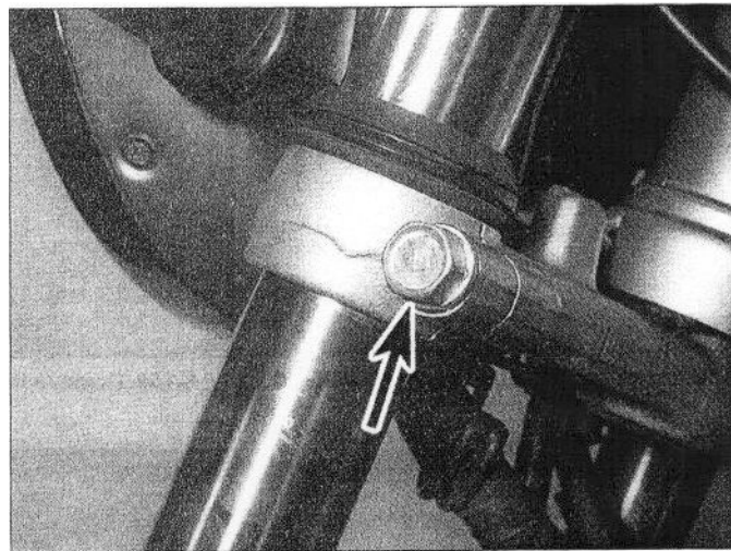
6.4b Bottom yoke fork clamp bolt (arrow)
