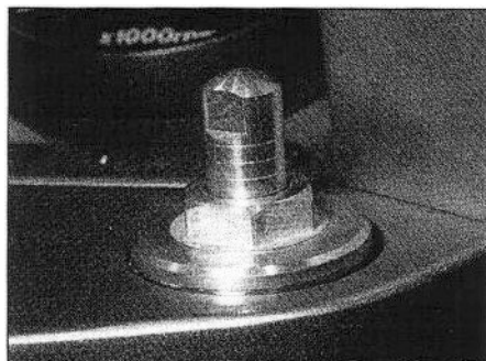
12.3 Front fork pre-load adjuster - UK N, P, R, S, T and V models (set to position 4)
