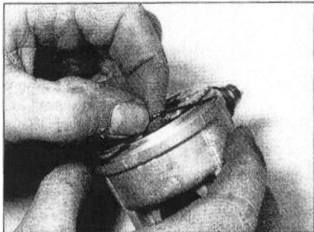
30.17 Fit a new O-ring around the cover
