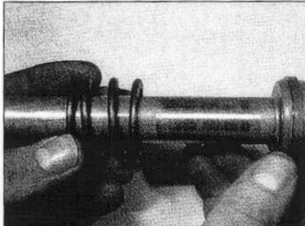
7.19a Slide the rebound spring onto the damper rod
