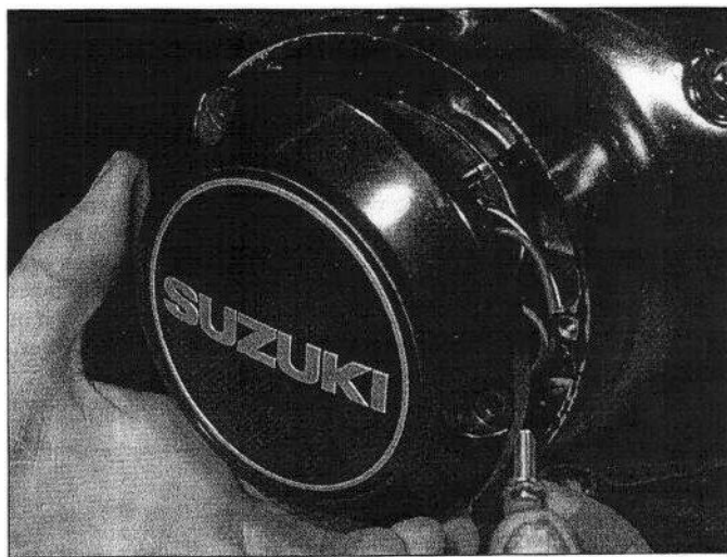
10.33 Install the pulse generator coil assembly cover
