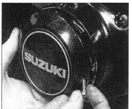
17.27 Install the pulse generator assembly cover
