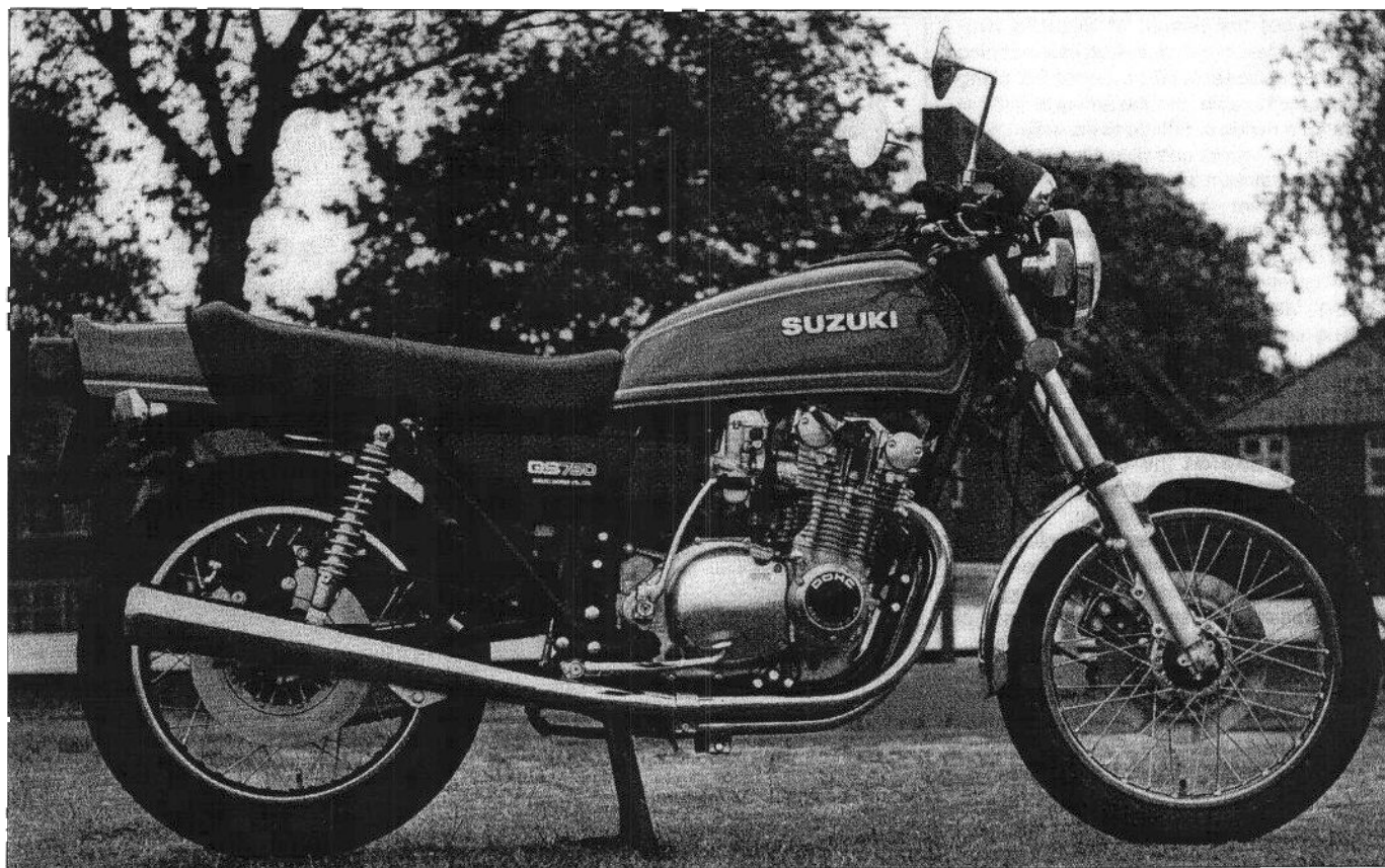
The 1976 GS750 – Suzuki's first four-stroke motorcycle
