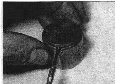
5.11a Prise the shim out of the follower (follower shown removed from engine) . . .
