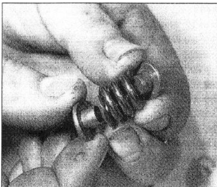
30.21c Fit the caps into the spring ends ...
