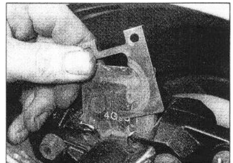
6.10a Make sure the anti-chatter shims are the right way round
