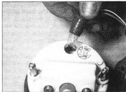
16.4b ... and remove the bulbholder
