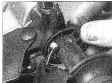
11.3b Detach the nipple from the lever
