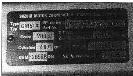
The identification plate is mounted on the right-hand side frame spar.
