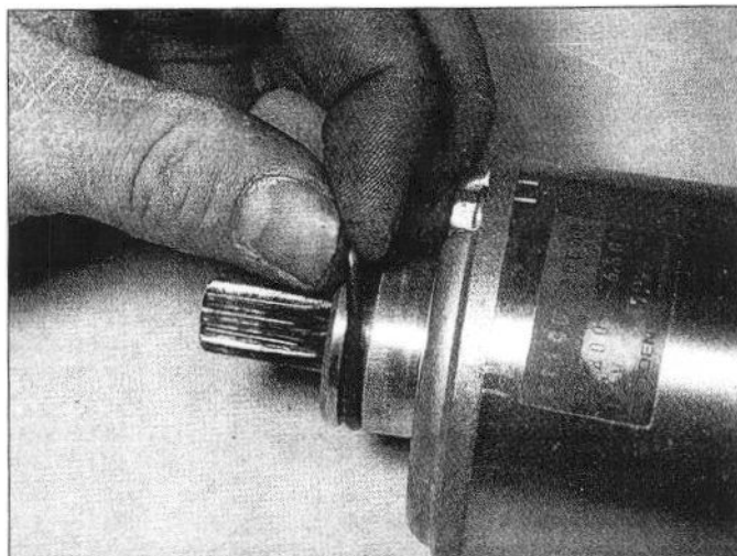
29.7 Fit a new O-ring onto the starter motor
