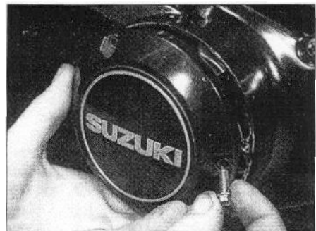
4.16 Install the pulse generator assembly cover
