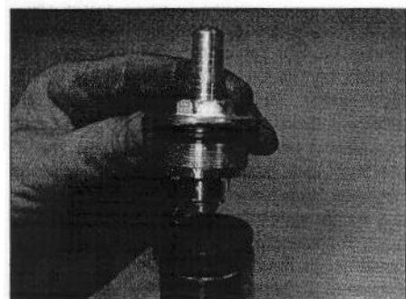
29.2 Unscrew the fork top bolt
