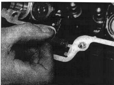
8.12 Lift the front camchain guide blade out of the engine
