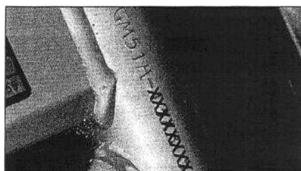
The frame number is stamped into the steering head right-hand side.
