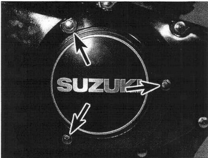
5.3 The pulse generator cover is secured by three bolts (arrows)
