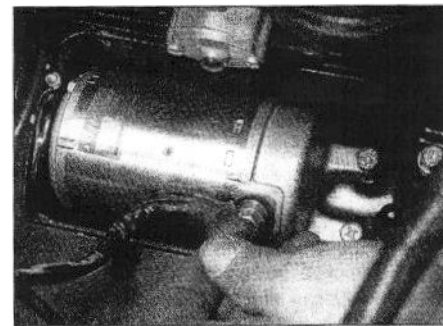
29.3 Peel back the cover to expose the terminal
