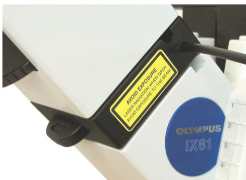
4: laser safety ocular shutter
