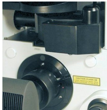
3: fluorescence turret and C-mount
