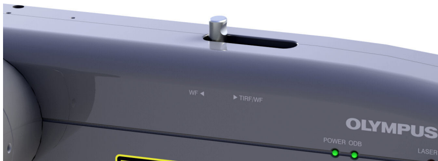
Light path selector slider. WF ◀ (left) : 100% widefield; ▶ TIRF/WF (right): 100% TIRF, 50% widefield
