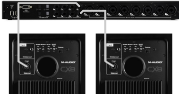
Audio Interface (Balanced TRS to Balanced TRS)
