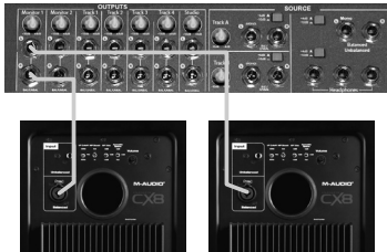
Control Room Router (Balanced TRS to Balanced XLR)
