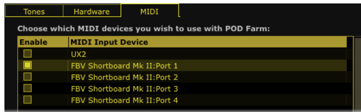
The Preferences, MIDI dialog - Selecting a MIDI Controller Device (Mac OS® X)*
