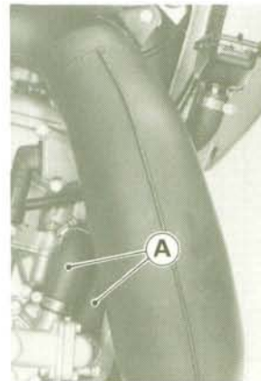
A. Cooling Hoses
