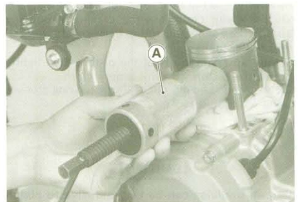
A. Piston Pin Puller Assembly: 57001-910
