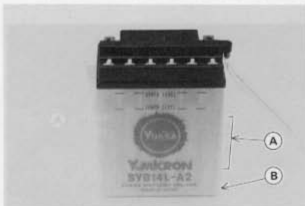
A. Sulfation here B. Sediment here
