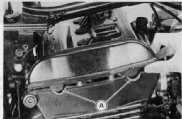
A. Apply silicone sealant here.
