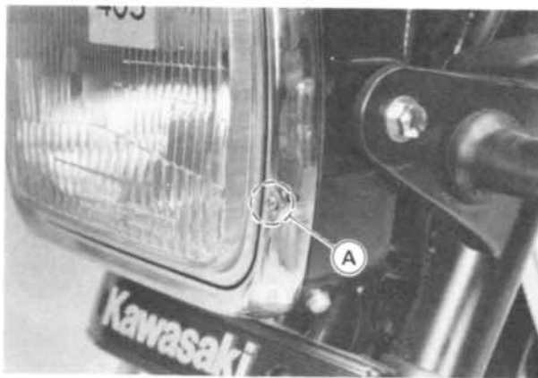
A. Adjusting screw for horizontal adjustment
