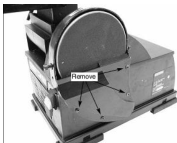
Figure 16 - Removing Disc Cover to Replace Disc
