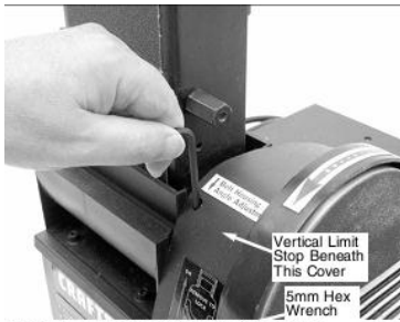
Figure 11 - Loosen Bolt to Tilt Self Assembly
