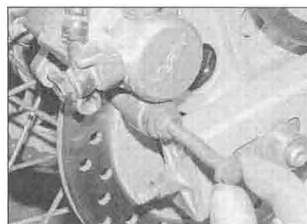
2.35c Install the bolt and tighten it securely
