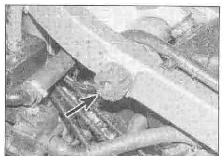
2.6 Check the mounting rubbers (arrow) for damage and deterioration
