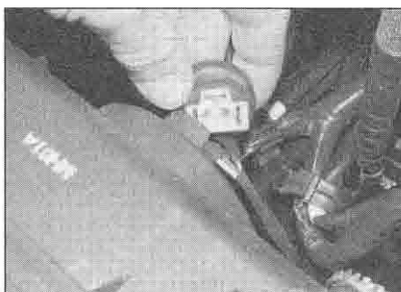
5.8c ... and disconnect the headlight wiring connector ...
