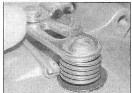
18.21d . . . and the spring ends locate correctly
