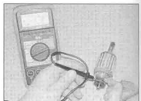
29.11 Continuity should exist between the commutator bars
