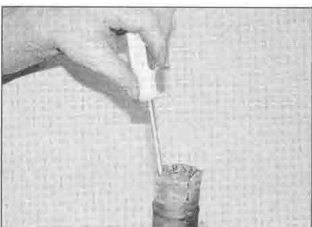
13.7a Dig out the old sealing ring ...
