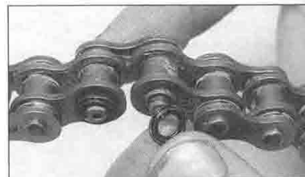
8.5 ... install the O-rings over the pin ends ...
