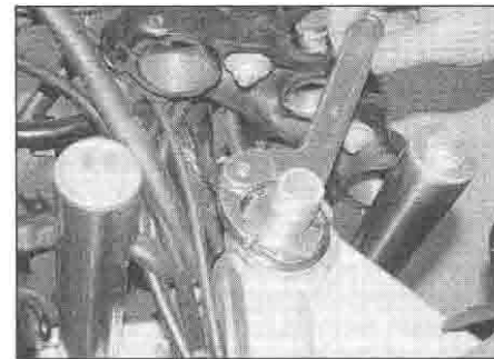
23.10 Adjust the bearings as described using either a C-spanner or a drift, or one of the special tools described
