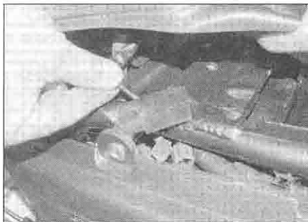
2.11b . . . and draw it out from under the frame rail
