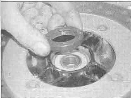
15.22 Fit the grease seal and press or tap it into place
