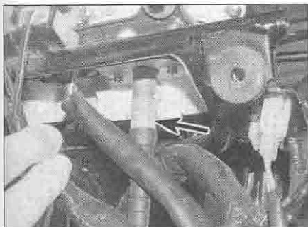
15.2 Unscrew the retaining ring (arrowed) and detach the cable
