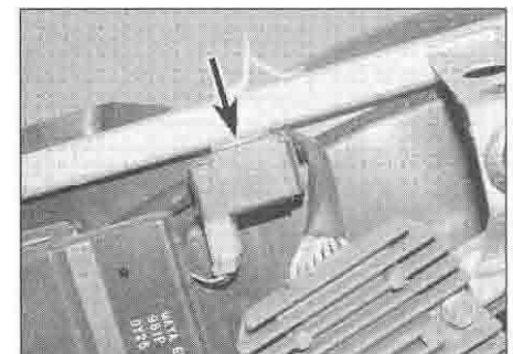
15.2c Fuel cut-off relay (arrowed) – XR750-P models onward
