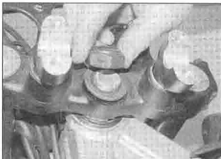
19.8b ... then unscrew the nut ...
