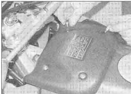
2.17a Undo the screws . . .
