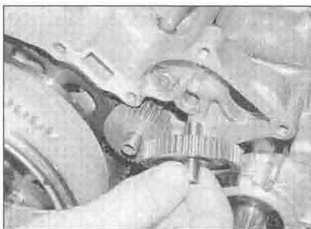
32.15b ... and the starter drive gear
