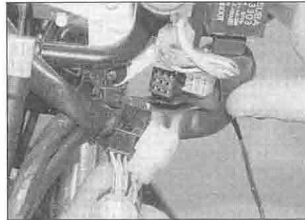
15.3b Instrument cluster wiring connectors – XL650V
