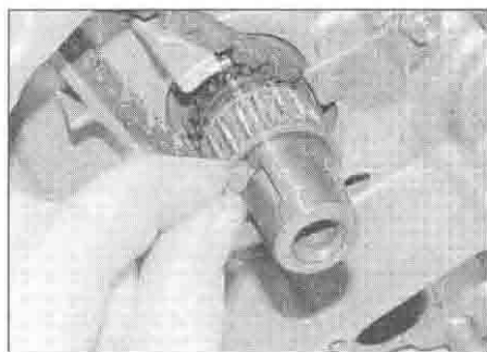
32.13 Fit the Woodruff key into its slot
