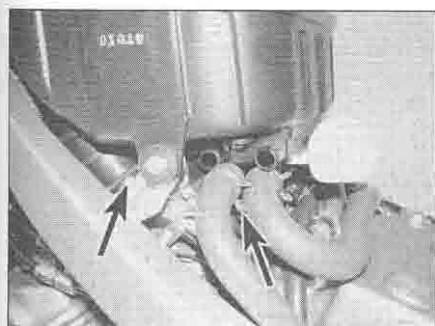
4.10 Slacken the clamp screws (arrowed)
