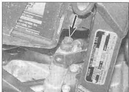
8.5 Brake hose banjo bolt (arrowed)
