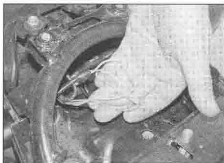
13.7 Rear turn signal wiring connectors – XL650V
