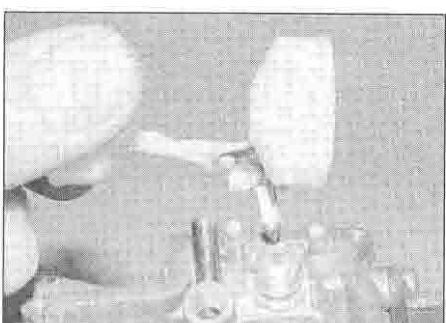
8.10b ... and remove the float assembly
