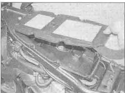
8.2c ... and lift out the filter
