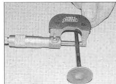
14.14a Measure the valve stem diameter with a micrometer . . .
