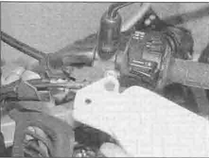
19.3c ... and remove the handguard
