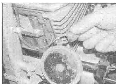
26.2 Disconnect the wiring connectors
