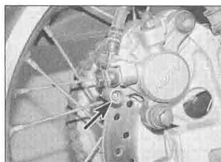
2.32b . . . then slacken the retaining pin (arrowed)
