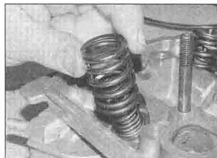
14.28b ... and the outer valve spring ...
