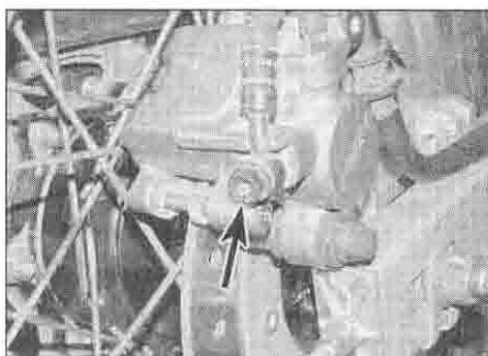
5.1a Brake hose banjo bolt (arrowed) – XL600V
