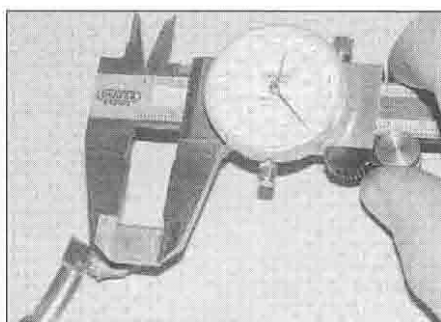
29.9 Measure the length of each brush
