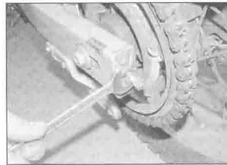
1.10b . . . and turn the adjuster as required until the slack is correct
