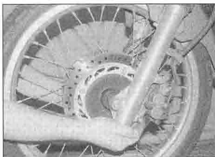
23.4 Checking for play in the steering head bearings
