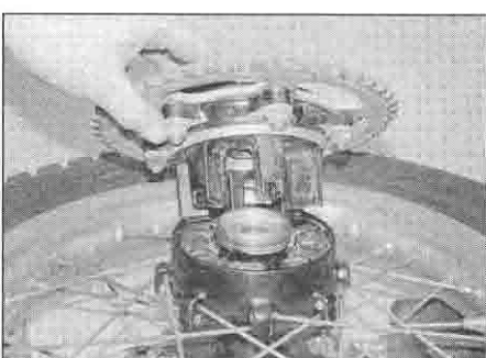
15.13 Lift the sprocket coupling out of the wheel
