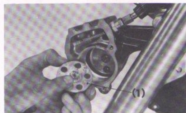
Fig. 4-24 (1) Applying silicon grease KS62M to pad B
