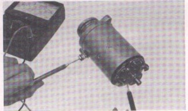
Fig. 5-24 Checking stator coil
