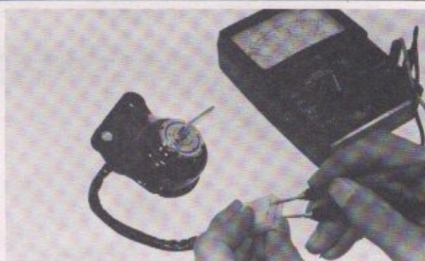
Fig. 5-29 Checking main switch for continuity
