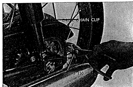
Fig. 4.83 Removing drive chain
