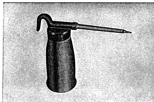
Fig. 6.47 Tools for chain lubrication
