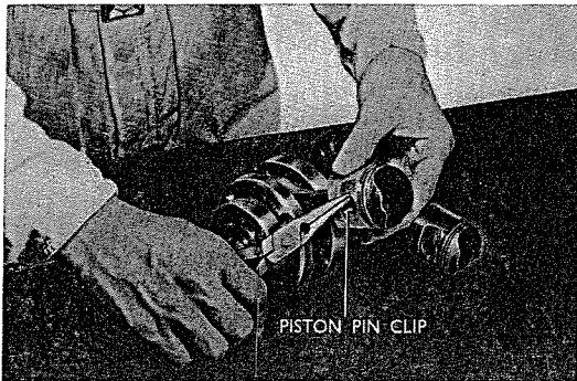
Fig. 3.95 Removing piston pin retainer
