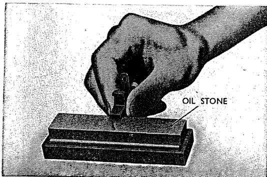
Fig. 5.24 Correction by oilstone
