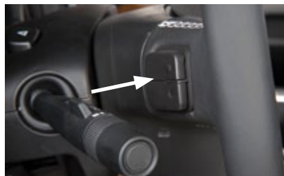
Next/Previous Favorite Station button shown. Volume button is located behind the right side of the steering wheel.
