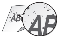
Toner smudges and splatters appear
