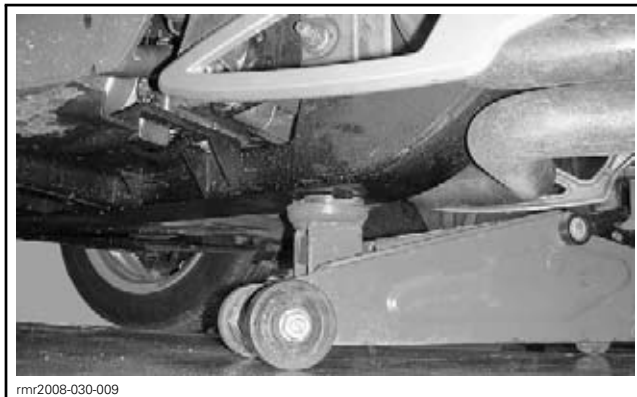
TYPICAL - LIFT BY THE FRAME
