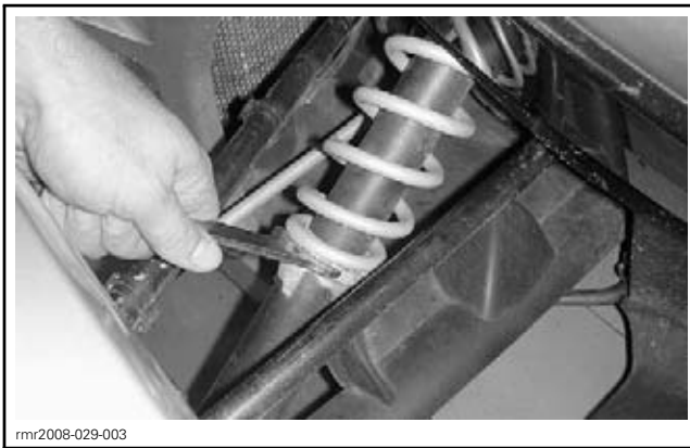
FRONT SUSPENSION CAM ADJUSTMENT
