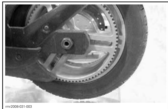
TYPICAL - SWING ARM ALIGNS WITH A SPOKE
