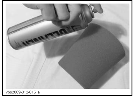
TYPICAL - SPRAY FOAM ELEMENT INSIDE AND OUT
