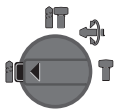
Position for drilling without impact in wood, metal, ceramic and plastic as well as for screwdriving
